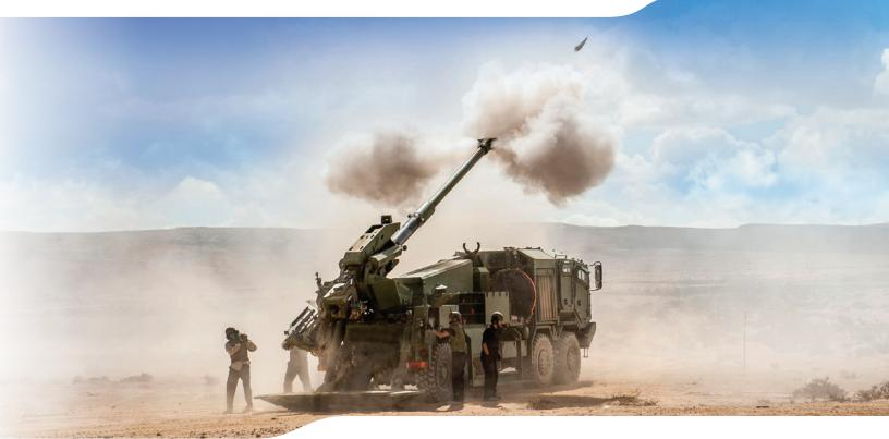
Elbit Systems' ATMOS is a 155mm/52 caliber truck-mounted howitzer that offers the advantages of superior fire power, enhanced mobility and rapid response time. Highly adaptable, the modular ATMOS system is compatible with any 6x6 or 8x8 high-mobility tactical truck. ATMOS supplies fire support for all types of missions and can be easily interfaced with customers' existing C<sup>4</sup>I systems.
